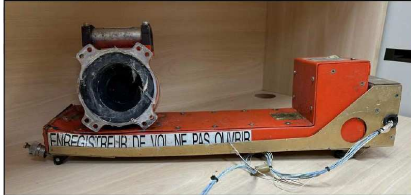
Figura 29 - Flight Data Recorder instalado na aeronave PS-VPB.
